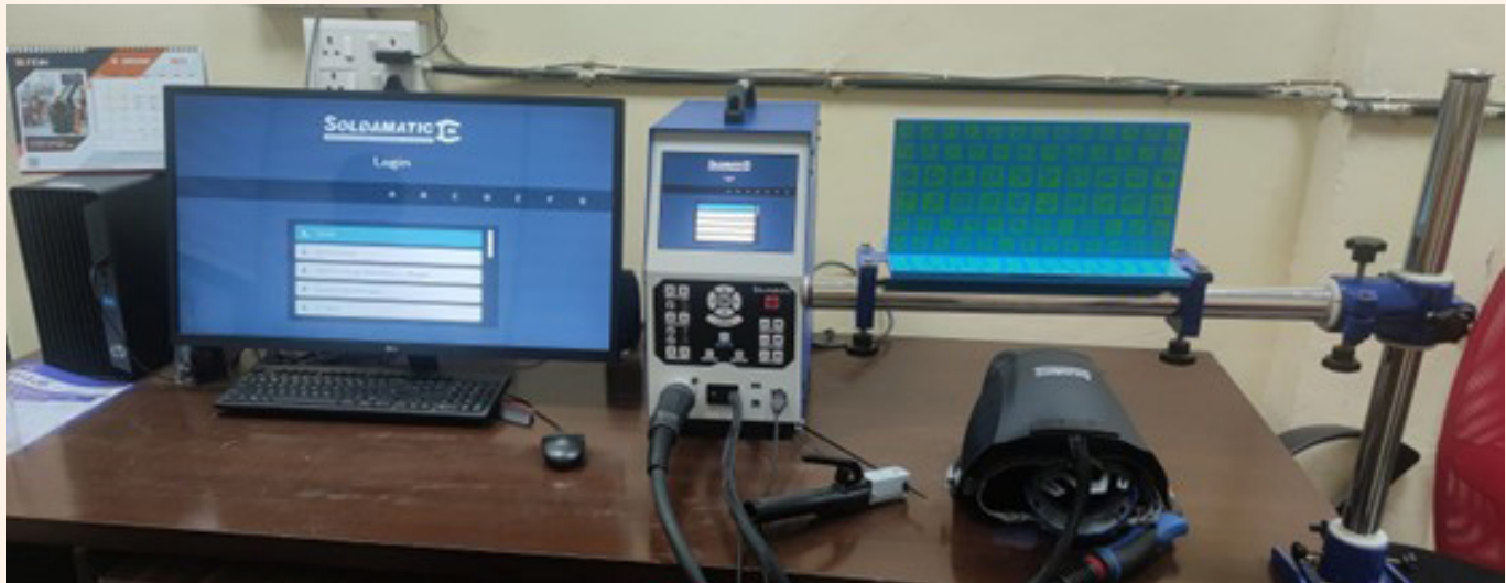
WELDING SIMULATOR SETUP
